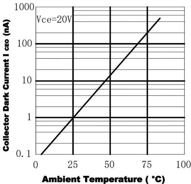
Fig.6 Collector Current vs.
