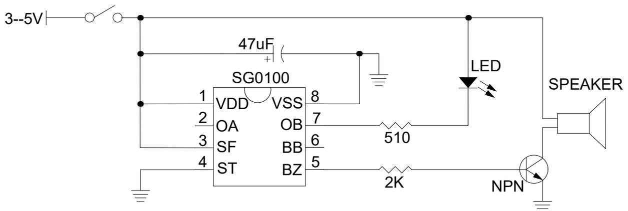
Application example 1: IC alarms when power is on, and stops when power is off. The circuit is simple and the quiescent current is zero.
