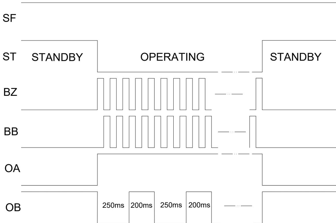
● **Pulse control mode timing diagram**
