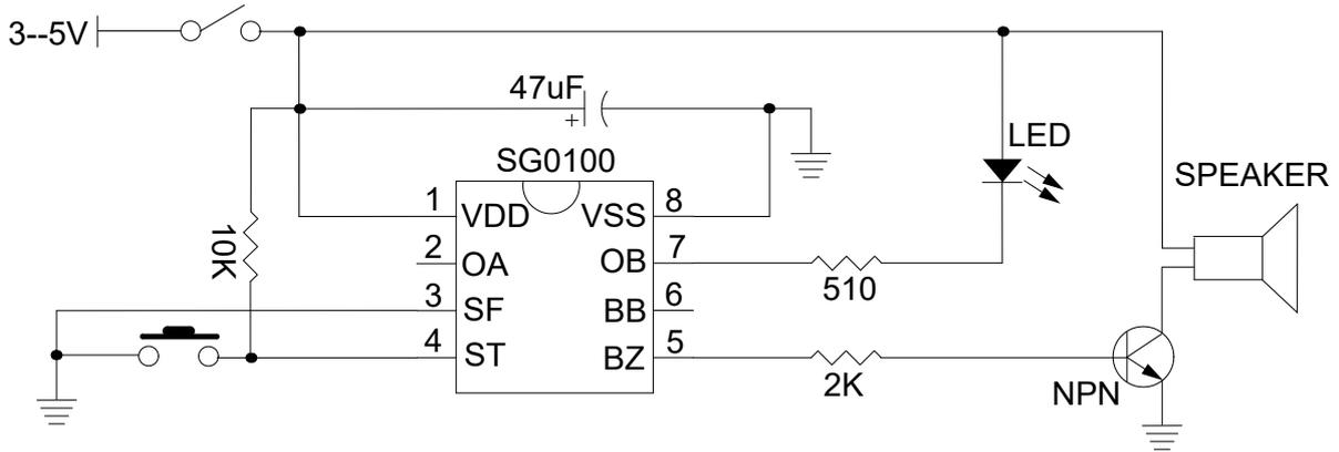
Application example 2: The IC is in the standby state after power-on, and alarms after S1 is triggered, and it can be stopped only when the power is turned off
